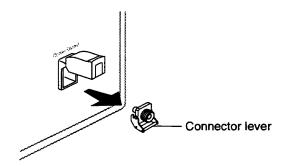
(3) Fit the new connector in the reverse procedure of removal. Take great care not to scratch or otherwise damage the connector or end face of the ferrule.
