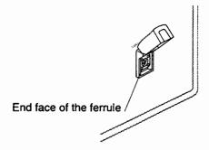
(4) Carefully refit the optical input connector taking care not to scratch or otherwise damage the end face of the ferrule.
